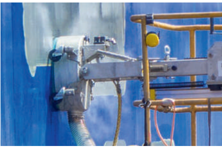
Preloaded springs ensure contact stability and gentle approaching
