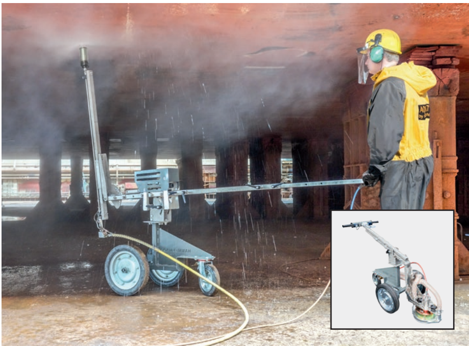
As a supplement to ceiling cleaning, an Aquablast is available for cleaning floors
