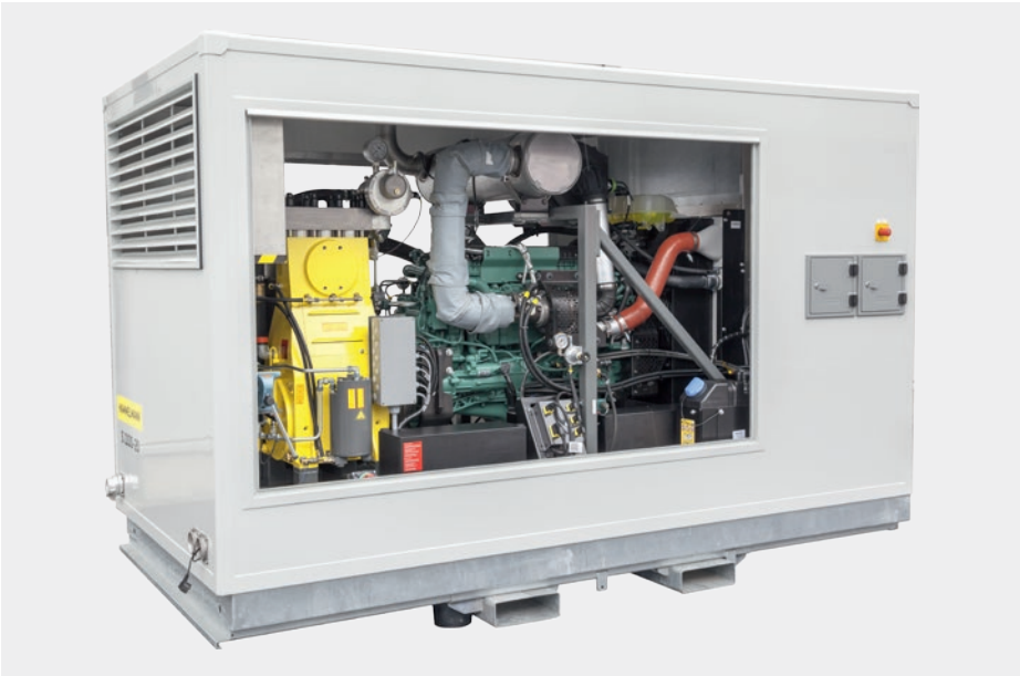
Stationary unit with sound damping cover
