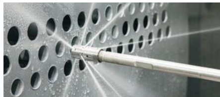
2nd gear – medium pump power i.e. for pipe and tube bundle cleaning
